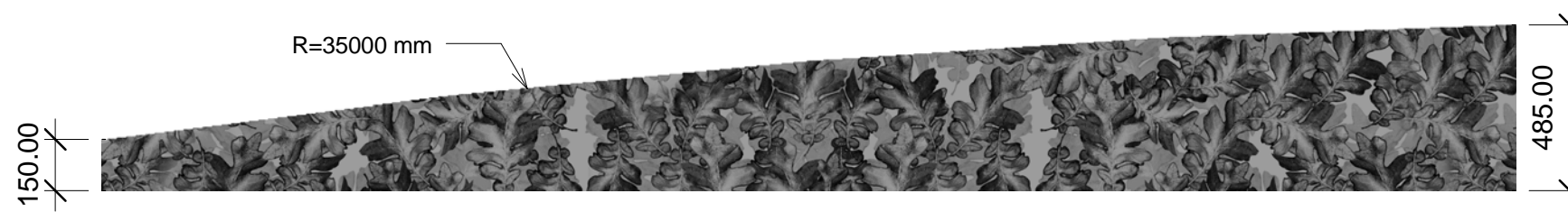
(front - top) Digitally printed vinyl protected with anti-graffiti, optically clear overlamine. Aluminum panel size: 4130mm x 485mm x 6.4mm
